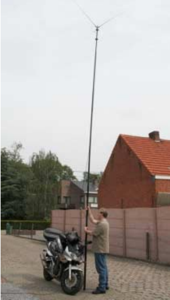
ON8PD setting up the 6M dipole XR-100 next to this motorcycle on a 25ft fiber pole
