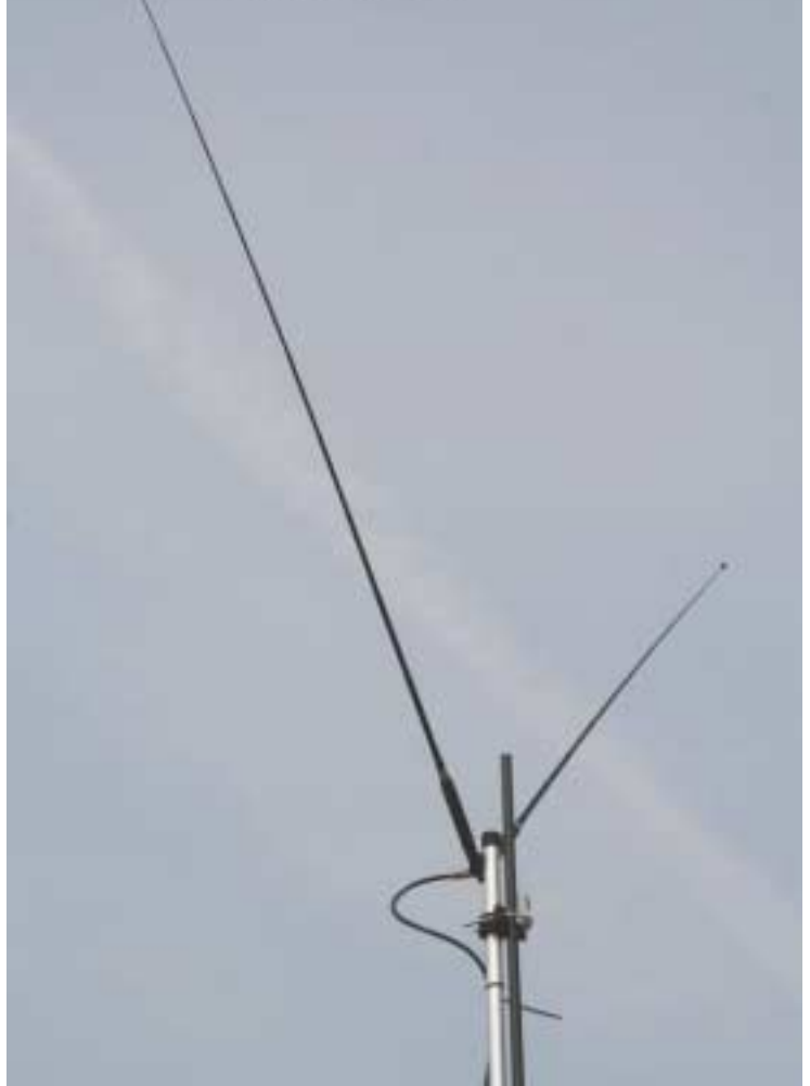
More close-up view of the XR-100 (with 20M coils) in the 25ft fiber pole.
