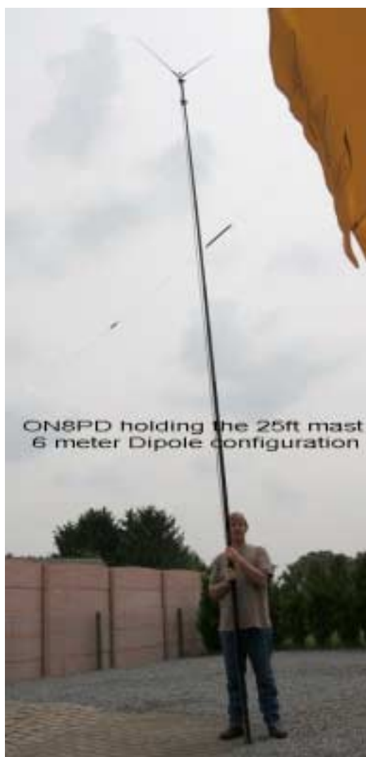
6 Meter configuration (2 telescopic whips only at 25 feet on 33ft telescopic fiber mast)
